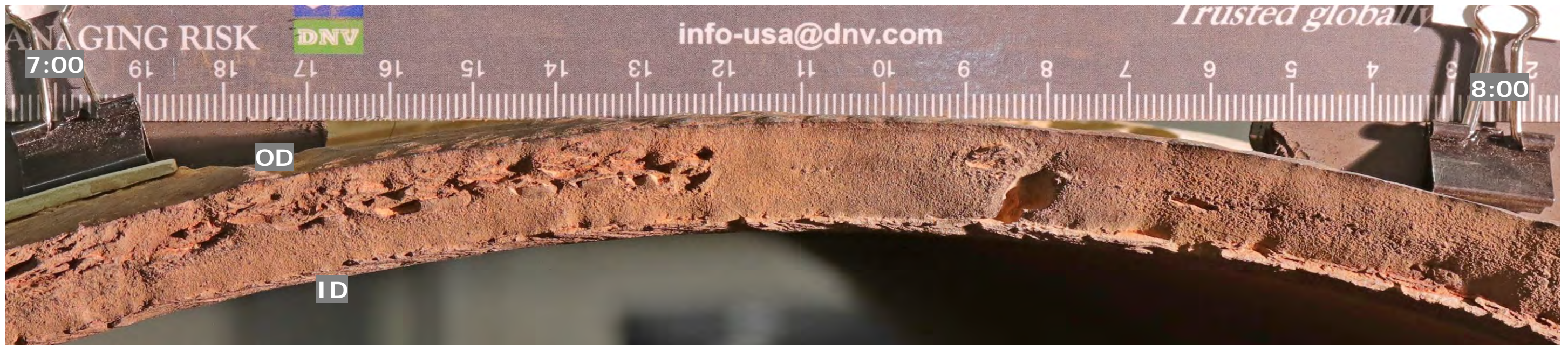
Figure 27. Photograph of the fracture surface of PS A between the 7 and 8 o'clock orientations. Units of ruler are in cm. Flow direction is into the photograph.
