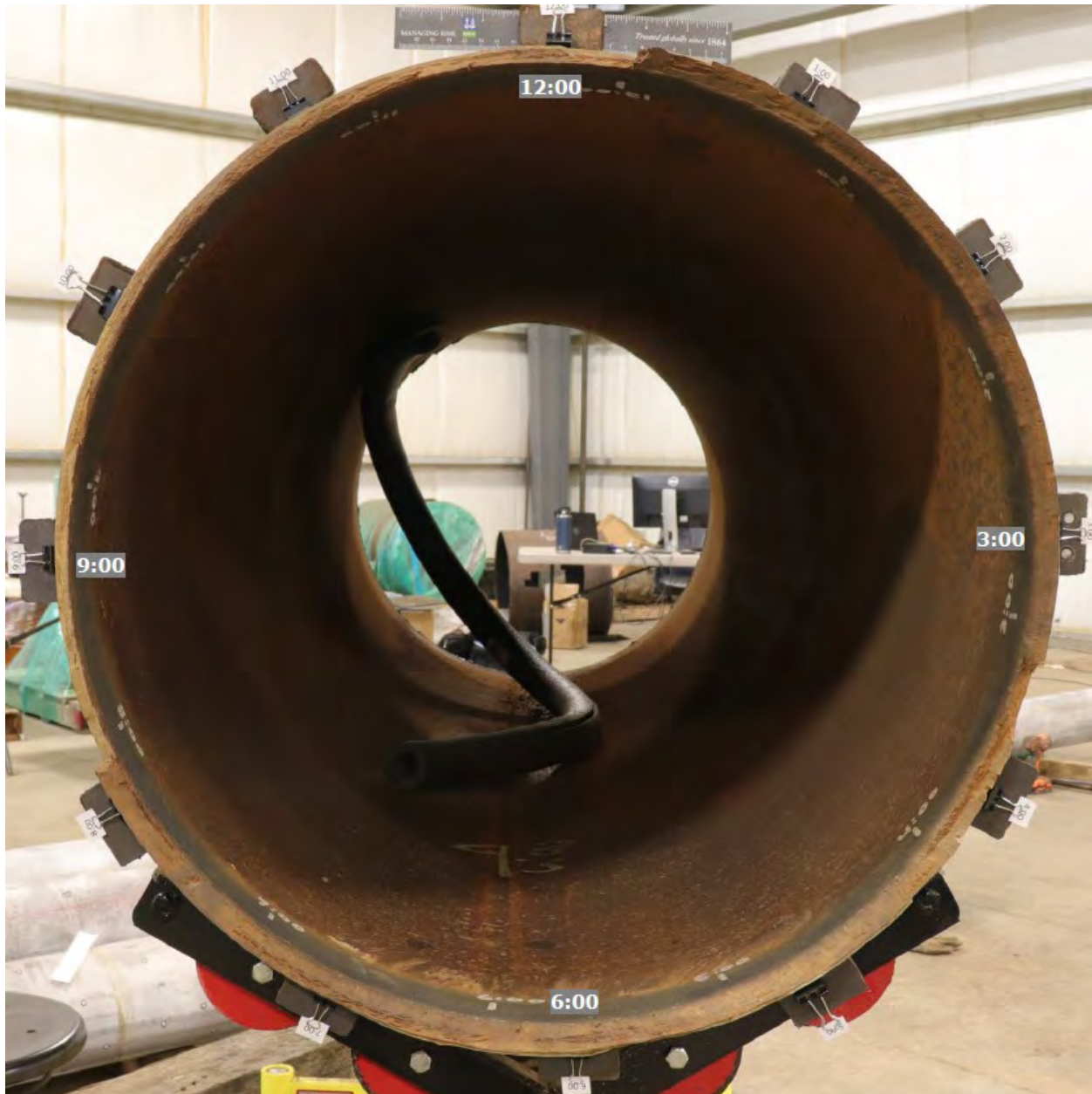
Figure 15. PS A Fracture Surface (Upstream to Downstream)
