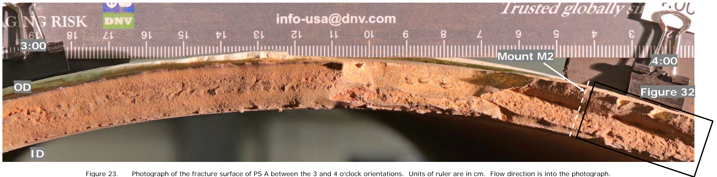
Figure 22. Photograph of the fracture surface of PS A between the 2 and 3 o'clock orientations. Units of ruler are in cm. Flow direction is into the photograph.
