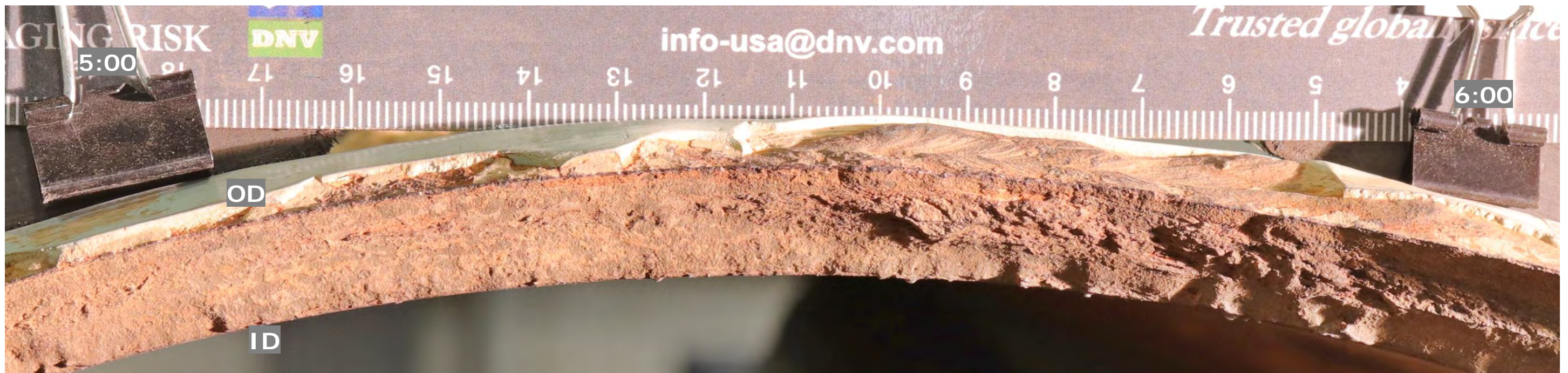
Figure 25. Photograph of the fracture surface of PS A between the 5 and 6 o'clock orientations. Units of ruler are in cm. Flow direction is into the photograph.
