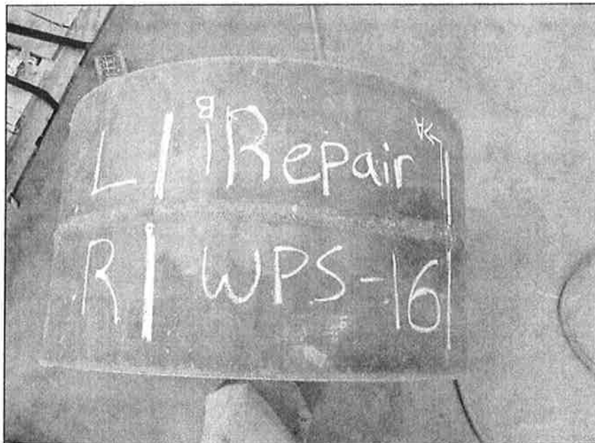
Figure 2. Typical completed girth weld coupon after cutting.
