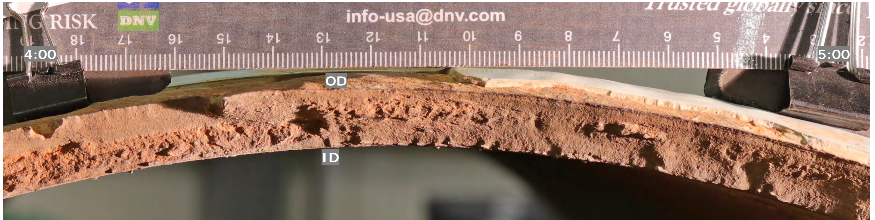
Figure 24. Photograph of the fracture surface of PS A between the 4 and 5 o'clock orientations. Units of ruler are in cm. Flow direction is into the photograph.
