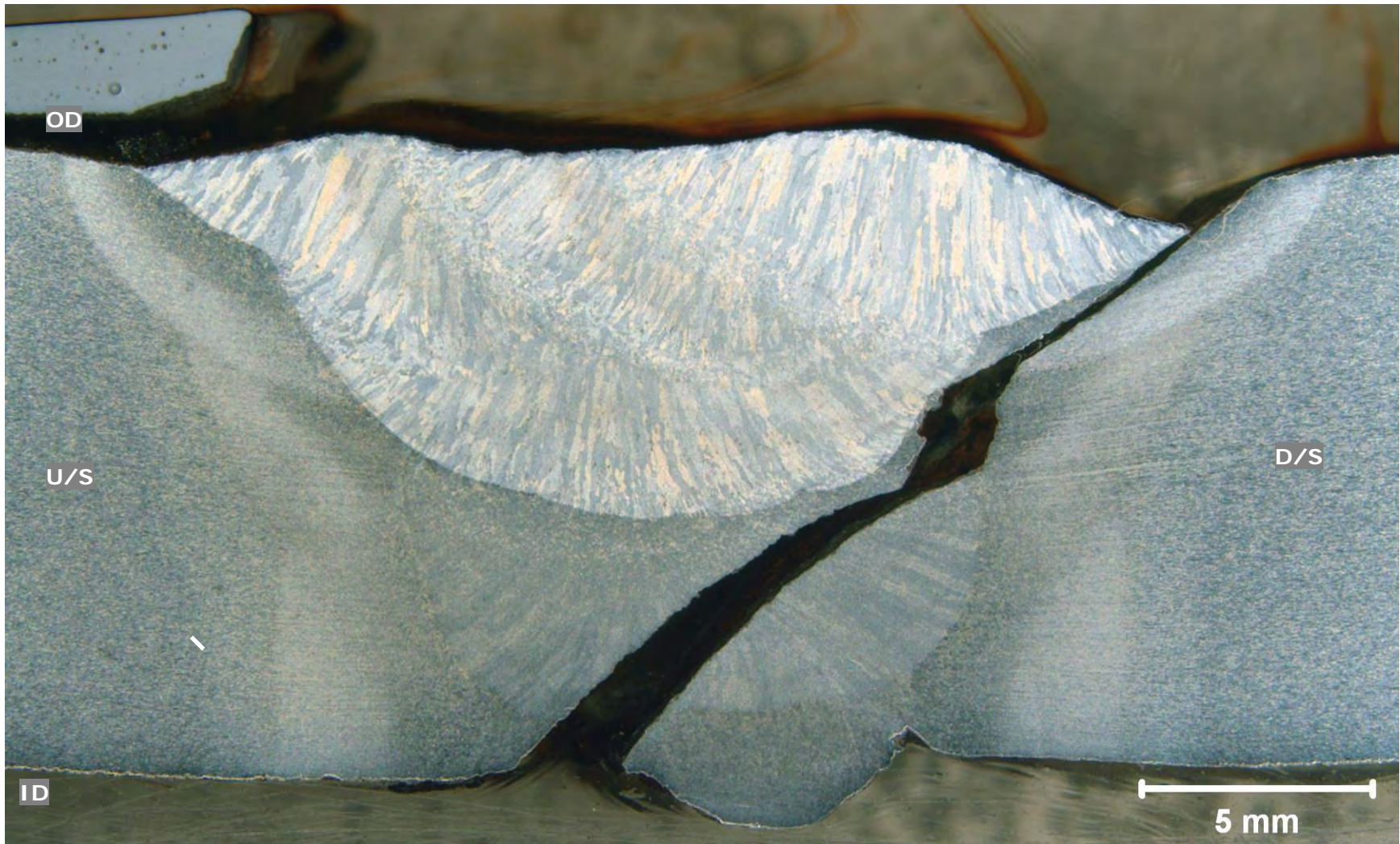
Figure 69. Light photomicrograph of Mount M5 (axial cross-section), which was removed from the GW at the 11:37 orientation; refer to Figure 1, Figure 14, and Figure 31 for location (2% Nital Etchant).
