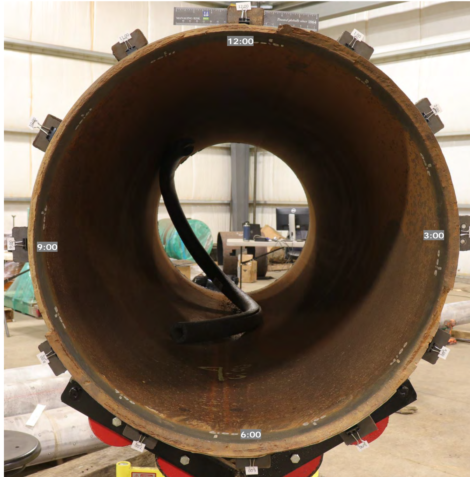
Figure 19. Photograph of the fracture surface and internal pipe surface of PS A. Flow direction is into the photograph. Labels on magnets indicate o'clock orientations.
