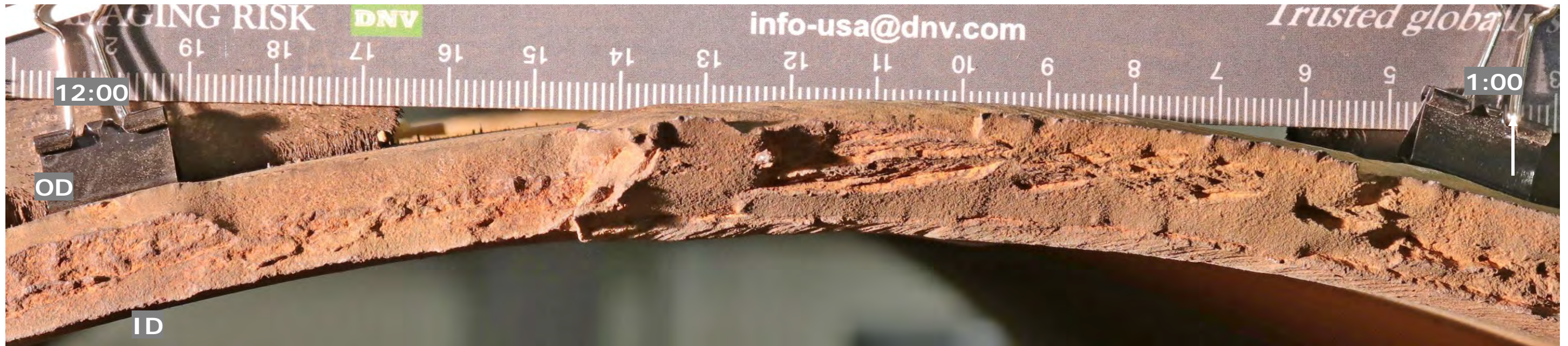
Figure 20. Photograph of the fracture surface of PS A between the 12 and 1 o'clock orientations. Units of ruler are in cm. Flow direction is into the photograph.
