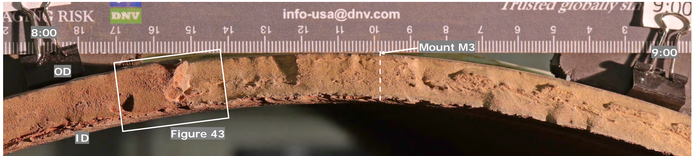
Figure 28. Photograph of the fracture surface of PS A between the 8 and 9 o'clock orientations. Units of ruler are in cm. Flow direction is into the photograph.
