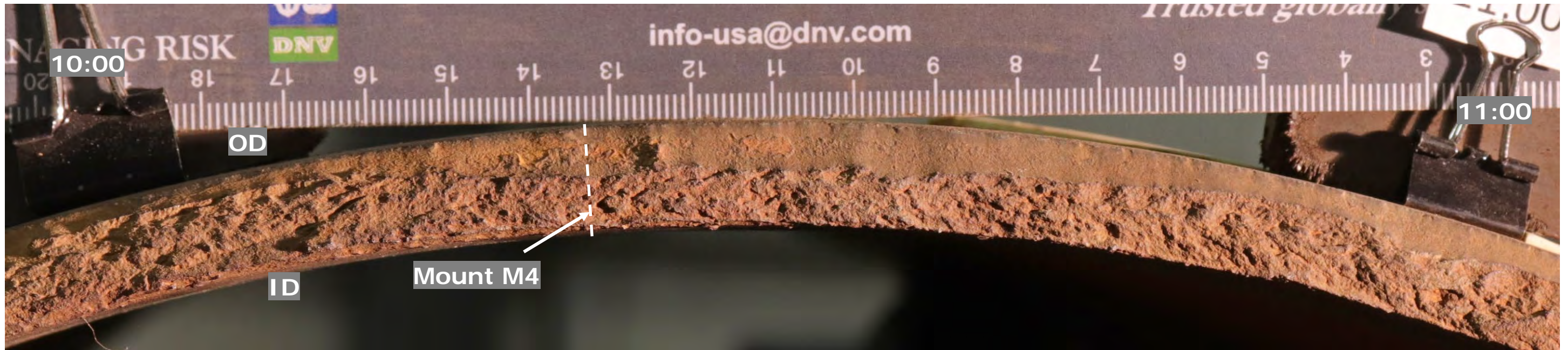
Figure 30. Photograph of the fracture surface of PS A between the 10 and 11 o'clock orientations. Units of ruler are in cm. Flow direction is into the photograph.
