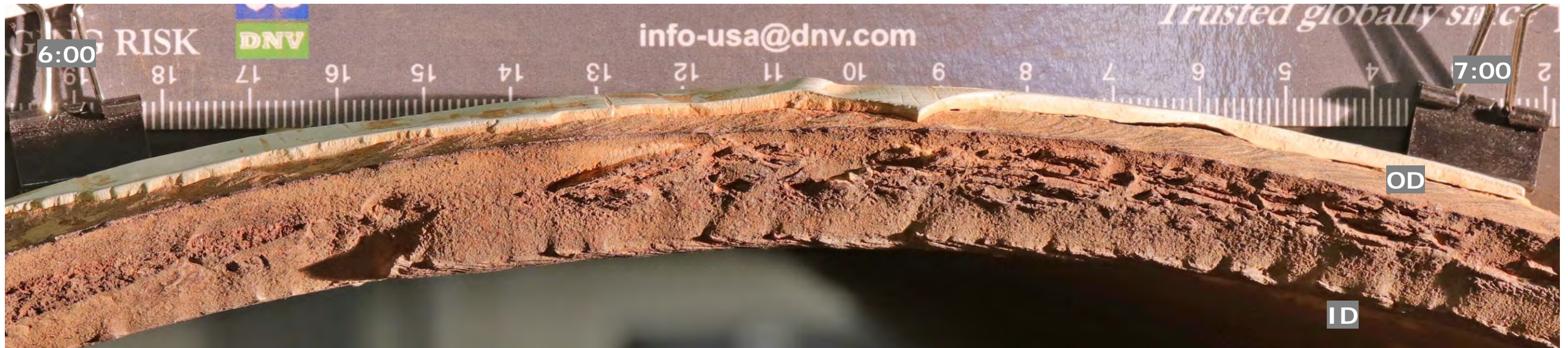
Figure 26. Photograph of the fracture surface of PS A between the 6 and 7 o'clock orientations. Units of ruler are in cm. Flow direction is into the photograph.
