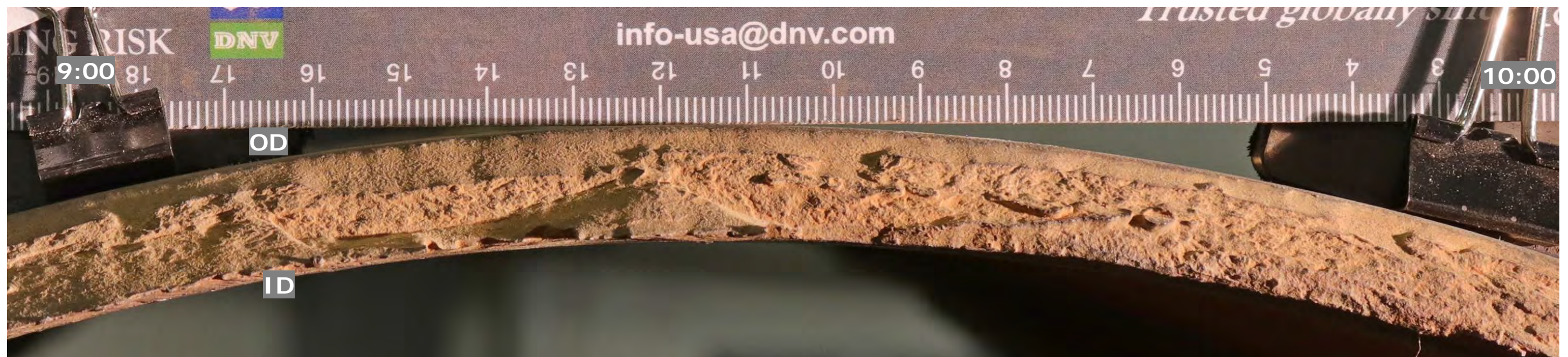
Figure 29. Photograph of the fracture surface of PS A between the 9 and 10 o'clock orientations. Units of ruler are in cm. Flow direction is into the photograph.
